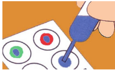
2. Apply a small drop of water in each circle. Don't touch the reagents
